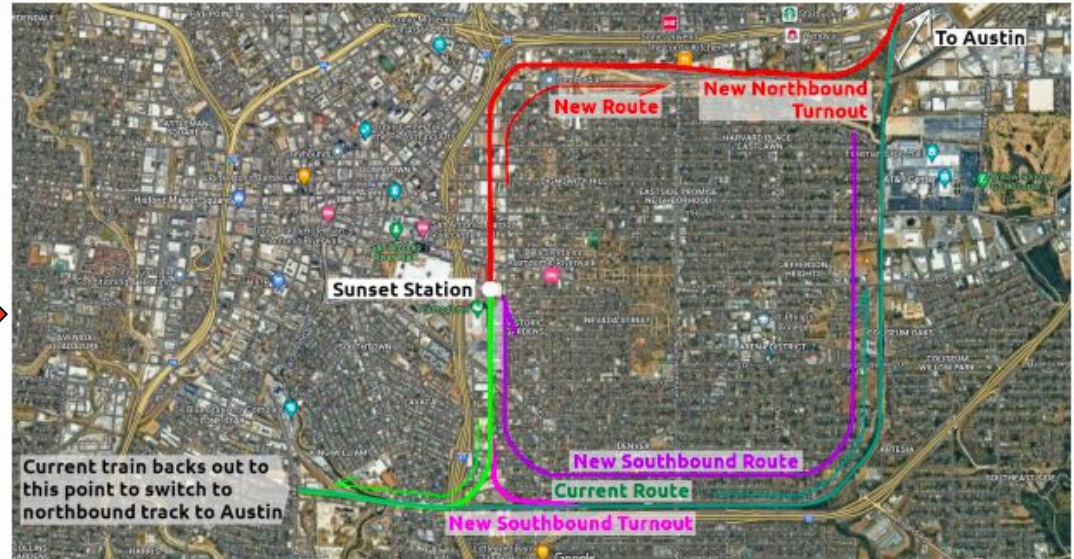
Figure 20: Current Texas Eagle back up maneuver and proposed new northbound and southbound routing, with new junction turnouts
